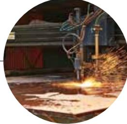
Energy efficient instruments such as inverter-based welding machines, plasma-cutting CNC machine, CO2 welding machines, and submerged arc welding machines are used in construction and repair activities.
